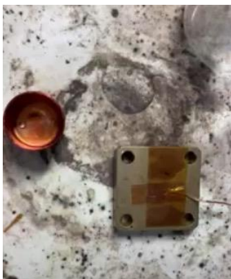
Image 2: Experiment station shown. Left: Copper cap. Right: thermocouple. Both objects are resting on the hot plate.
