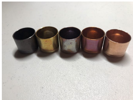
Image 3: Color differences between copper caps. The newest cap is on the right while most used is on the left. Caps in between follow the gradient order.
